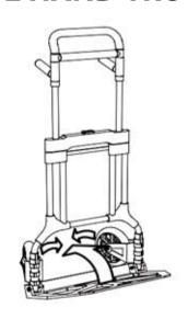
STEP 1: **FOLD NOSEPLATE UPWARD AND WHEELS WILL NEST INWARD AUTOMATICALLY.**
