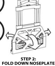
**FOLD DOWN NOSEPLATE** AND WHEELS WILL **AUTOMATICALLY EXTEND OUTWARD.**
