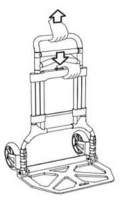
STEP 3: **PUSH BUTTON ON** CROSSBAR AND PULL UP HANDLE TO EXTEND.
